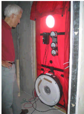
Fig. 2.3.1: Blower Door test in an apartment.
